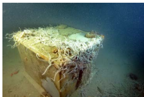
Fig. 2 : incubation chamber after 10 months at 27 m depth in the northern Adriatic Sea.
