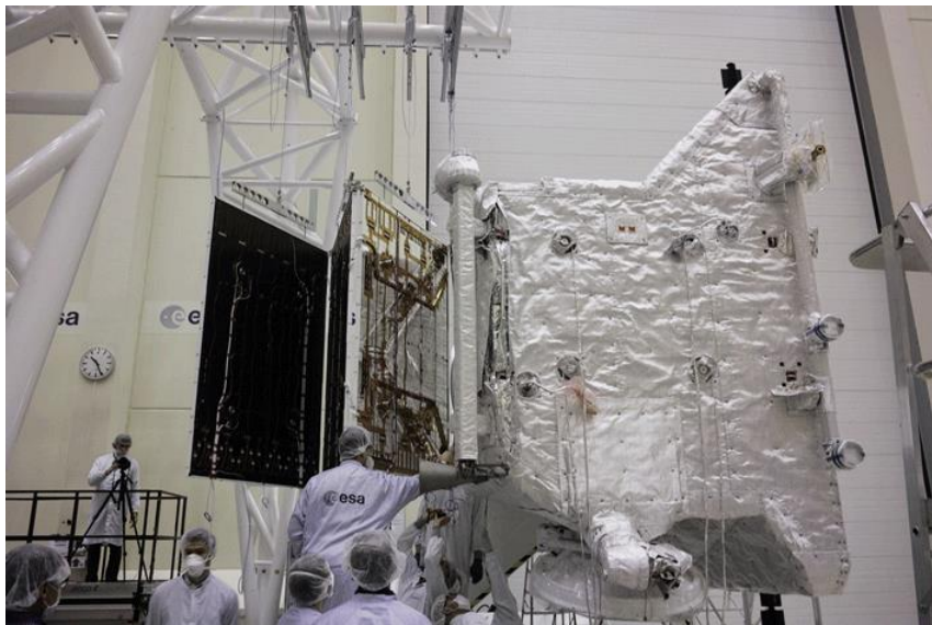
BEPICOLOMBO SOLAR WING DEPLOYMENT TEST
